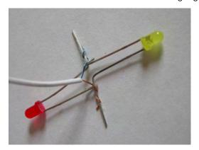
Solder the wires to the resulting leg connections.
