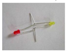
Flip one of the LEDs around, and connect the LED "Long leg > Short leg"
